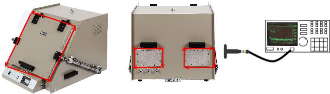
Figure 6-4 Measuring Maximum Leakage (ex. value: -90 dBm)
