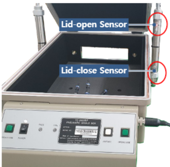
Figure 4-5 Lid-open/close Sensor Locations
