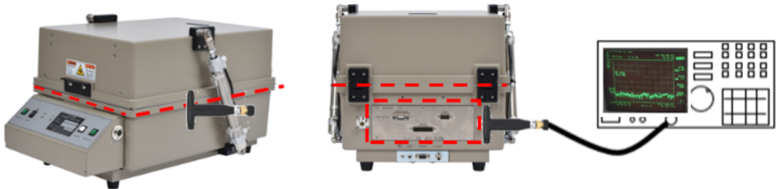
Figure 6-4 Measuring Maximum Leakage (Ex. Value: -90 dBm)
