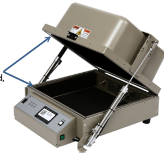
Figure 6-1 TC-5916AP Gasket Placement
