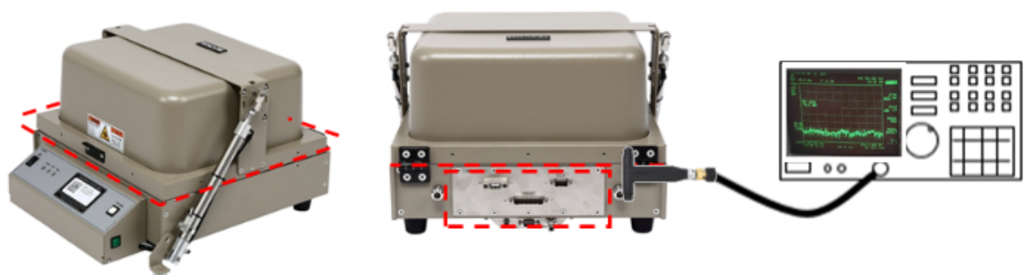
Figure 6-4 Maximum Leakage Test (Ex, value : -90 dBm)
