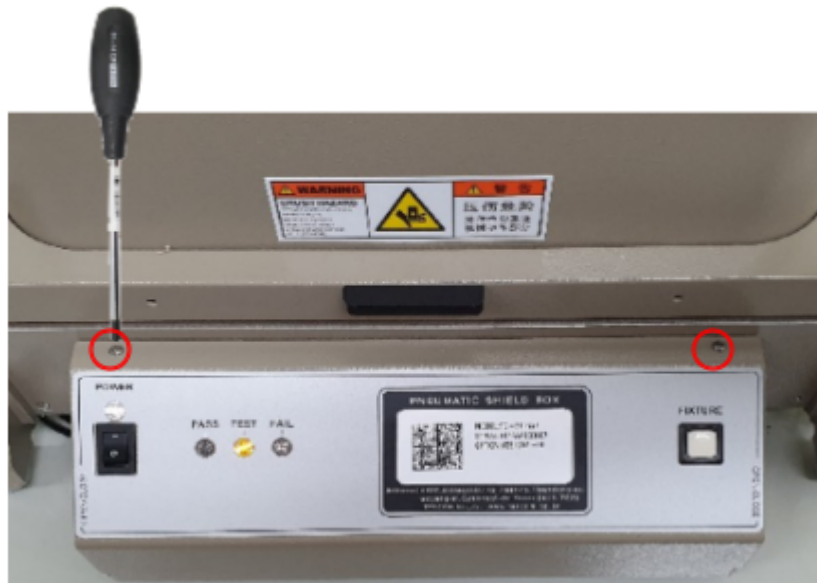
Figure 4-5 Control Box Open
