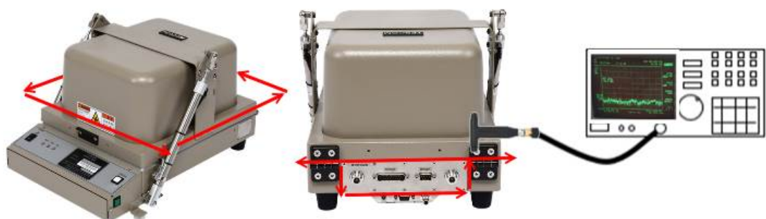
Figure 6-4 Measuring Maximum Leakage (Ex, value : -90 dBm)
