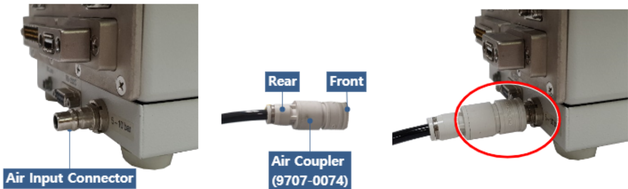
Figure 4-4 Connecting/Disconnecting compressed air supply
