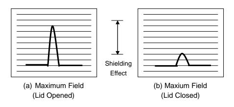
[Figure 12] Spectrum Analyzer Display
