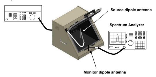
[Figure 11] Shielding Measurement Test Set Up (ex : TC-5970C)
