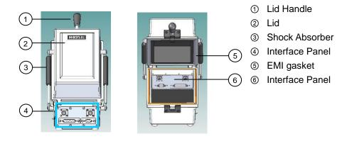
[Figure 1] TC-5910D Component Identification
