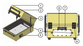
[Figure 5] TC-5922A Component Identification
