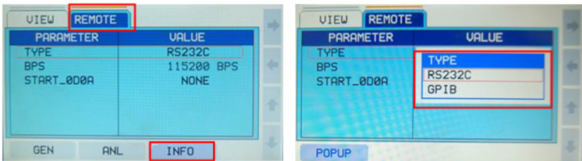
Figure 12-2 Remote Interface Setting Screen
